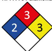
Note: The hazard category numbers found in GHS classification in section 2 of this SDSs are NOT to be used to fill in the NFPA 704 diamond. Blue = Health, Red = Fire, Yellow = Reactivity and White = Special (Oxidizer or water reactive substances)
