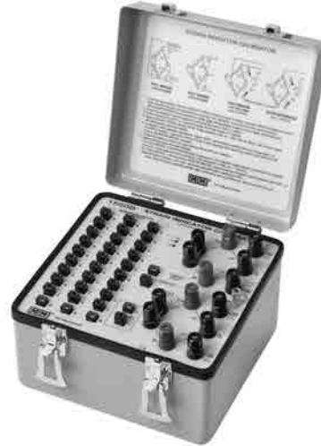
A laboratory standard for verifying the calibration of strain and transducer indicators.
