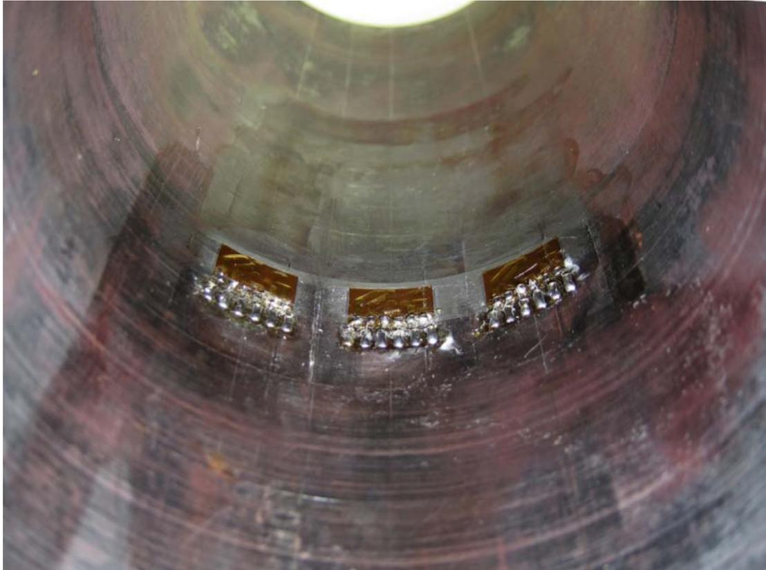
*Figure 1: Photograph showing three hole-drilling strain gage rosettes installed on the pipe's inner diameter*
