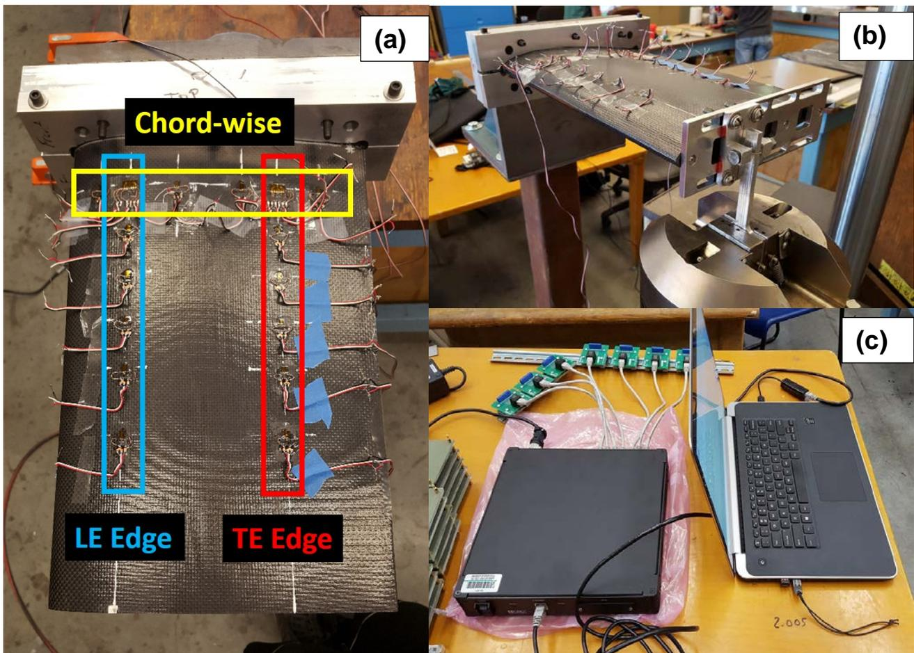
Figure 1: (a) Composite wing model with strain gages applied to the top skin surface. (b) Composite wing with strain gages mounted in the rigid fixture and Instron machine before fatigue testing. (c) System 8000 DAQ connected to a laptop for data collection from strain gages during testing.
