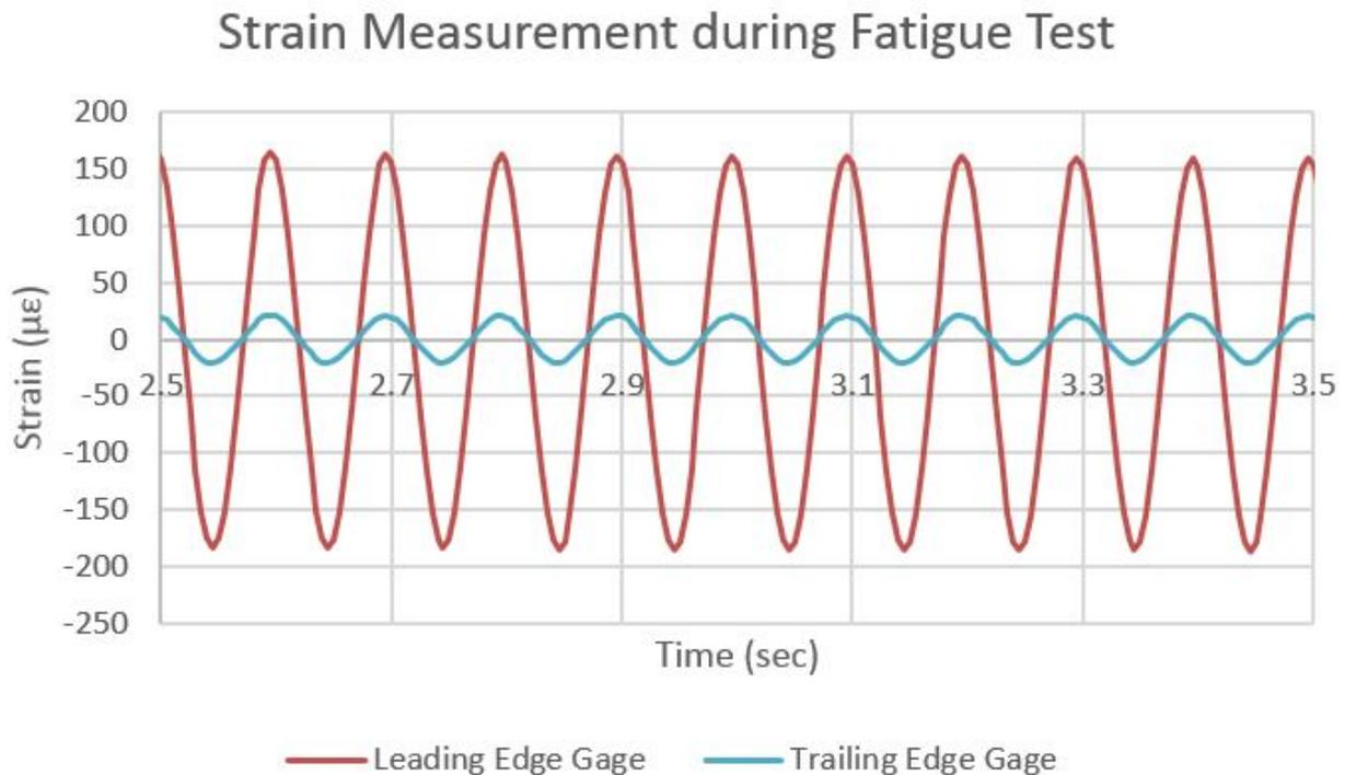
*Figure 3: Strain data at leading and trailing edge during fatigue test.*
