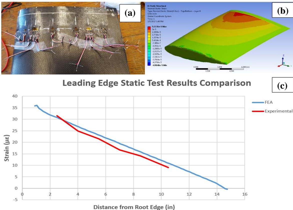
Figure 4: (a) Strain gages along the chord wise direction. (b) Strain contour plot from the FEA software. (c) Experimental and FEA strain results along the leading edge spar.
