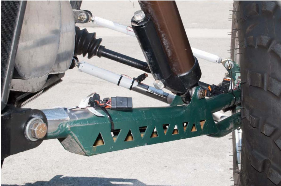
Figure 3: Rear suspension outfitted with strain gages on linkages, trailing arm and integrated upright. All gages are sealed with RTV and covered with thermal reflecting tape.
