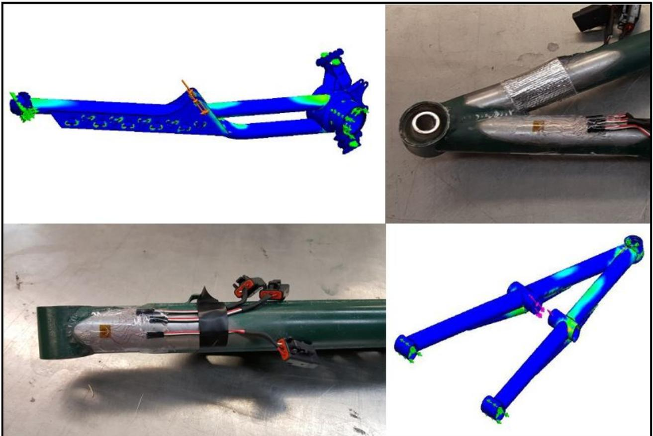
*Figure 2: FEA model of trailing arm (top left). Stacked rosette applied to trailing arm (bottom left). Lower A-arm with a stacked rosette applied to each side with one covered by thermal reflecting tape (top right). FEA model of lower A-arm (bottom right).*
