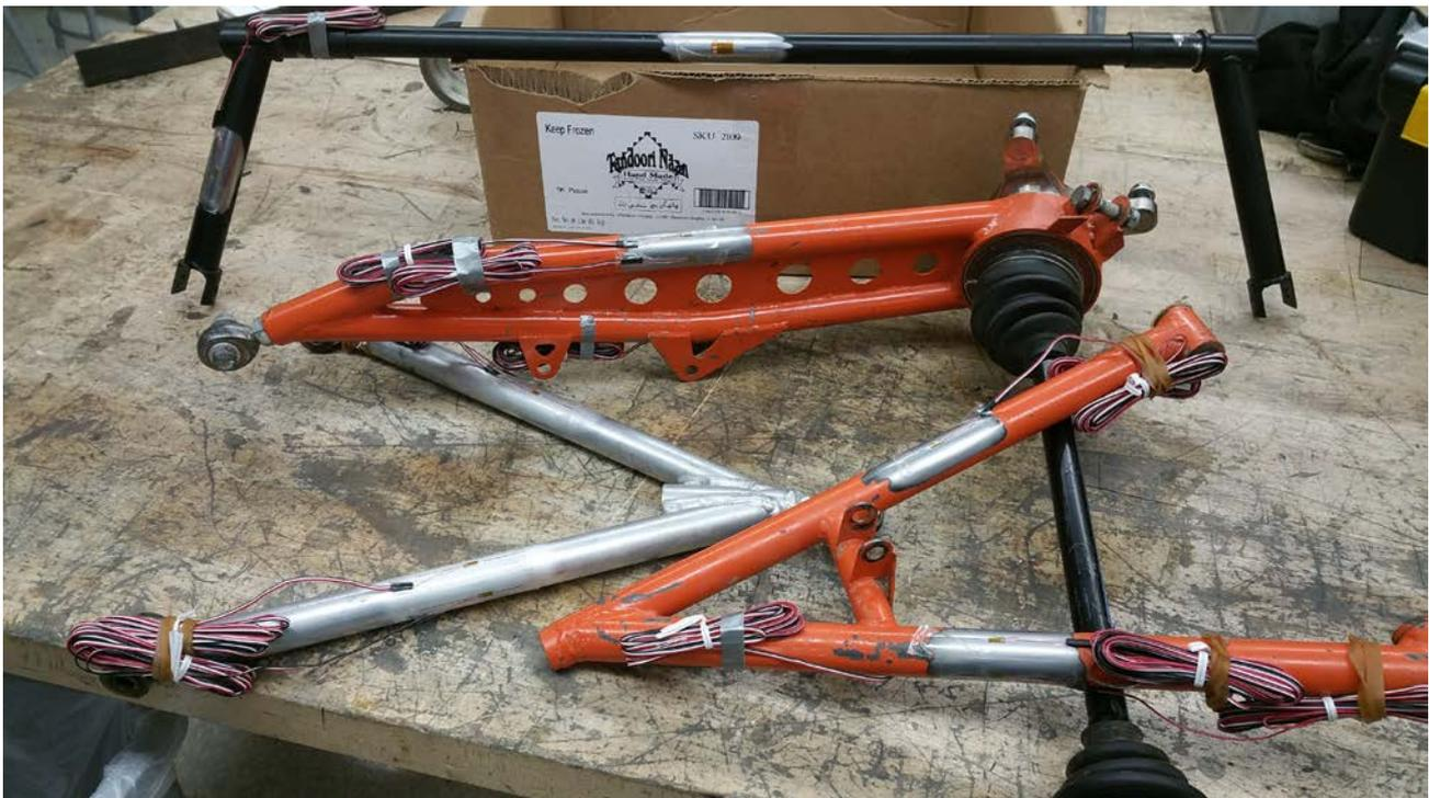
*Figure 1: Gaged and Calibrated Suspension Components Ready for Testing*
