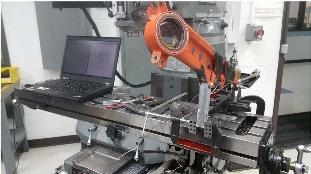
*Figure 2: Trailing Link Calibration by Hanging Calibrated Weight Sets*
