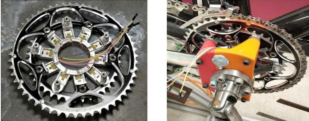
Figure 3: Sensor member retrofitted with the existing crankset
