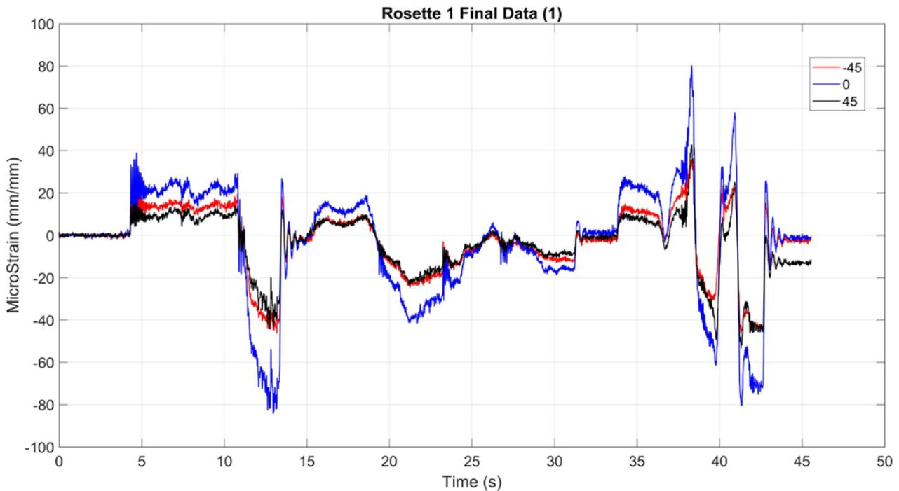
*Figure 1: Sample data from one rosette through dynamic testing*
