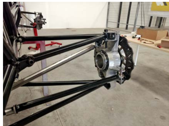
Fig. 2 Front view of a part the car showing suspension arms
