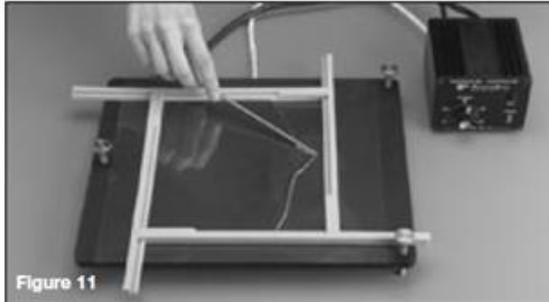
If air bubbles are present, wait a few minutes and burst them with a dental probe or a similar pointed object. Replace the cover over the casting plate.
