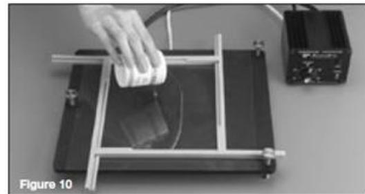
DO NOT scrape excess plastic from the cup sides and bottom onto the casting plate, as these are areas where a non-uniform mix is most likely to occur. As illustrated in Figure 11 on page 6, the stem thermometer or a wooden tongue depressor may be used to help spread the plastic over the entire plate surface (the liquid will level with time). Place the cover over the poured sheet to protect it from dust and other foreign matter during polymerization and switch the temperature controller off.
