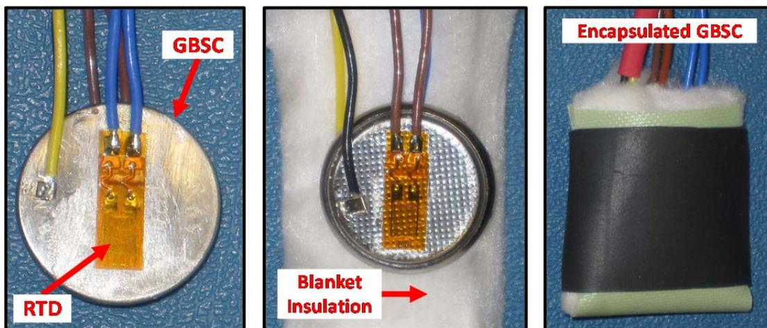
Figure 1: Assembly process for encapsulating the GBSCs
