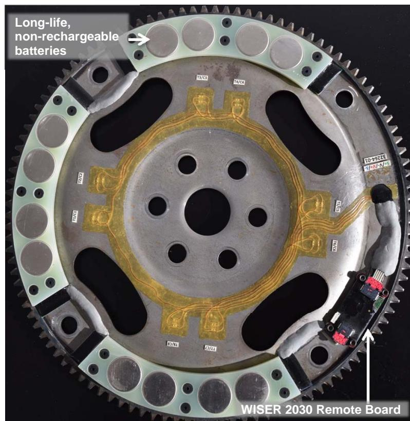
Figure 2: Sample Torque Sensing Flex Plate
