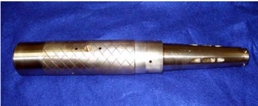
*Figure 1: Hybrid force balance*
