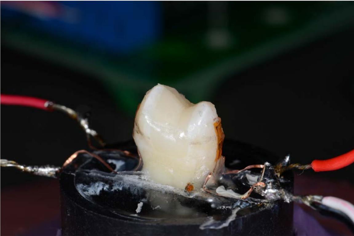
Figure 1: Micro-Measurements model EA-06-062AP-120/LE strain gages bonded to a maxillary premolar. The gages are connected to a D4 data acquisition conditioner.
