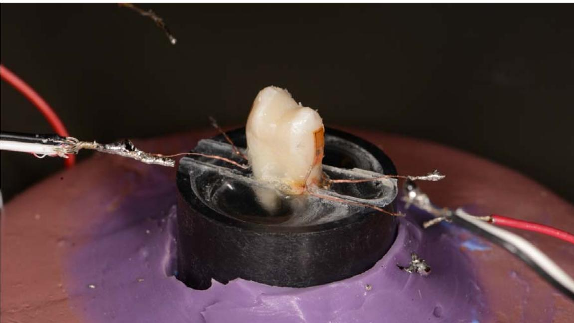
Figure 2: Maxillary premolar mounted in a phenolic ring with Micro-Measurements model EA-06-062AP-120/LE strain gages bonded.
