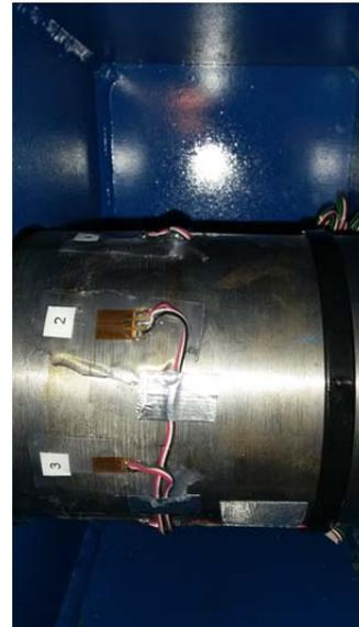
Picture 5: Strain gages installed on the reclaimer screw shaft: two full-bridges in shear patterns (torque) and two half-bridges in linear patterns (bending)
