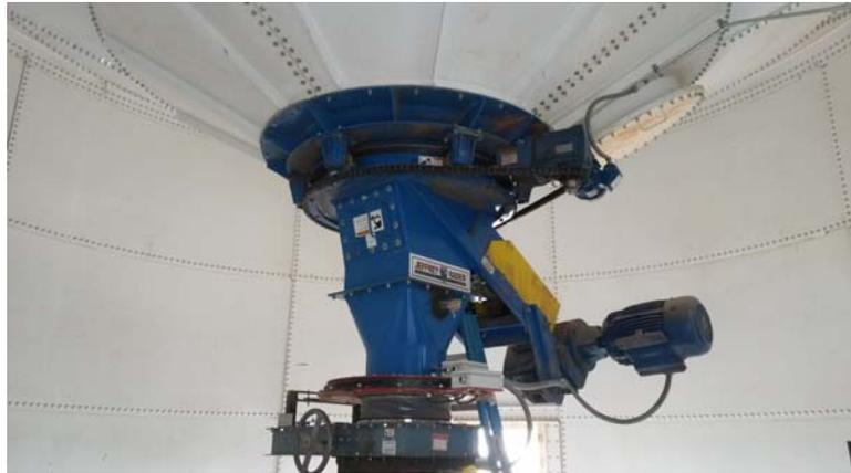
Picture 2: Reclaimer screw system installed at the bottom of the silo
