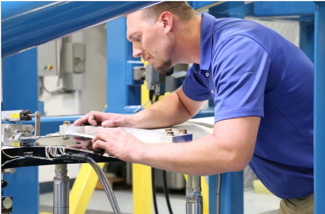
*Image 2: Inspecting strain gages on fatigue test blade section*
