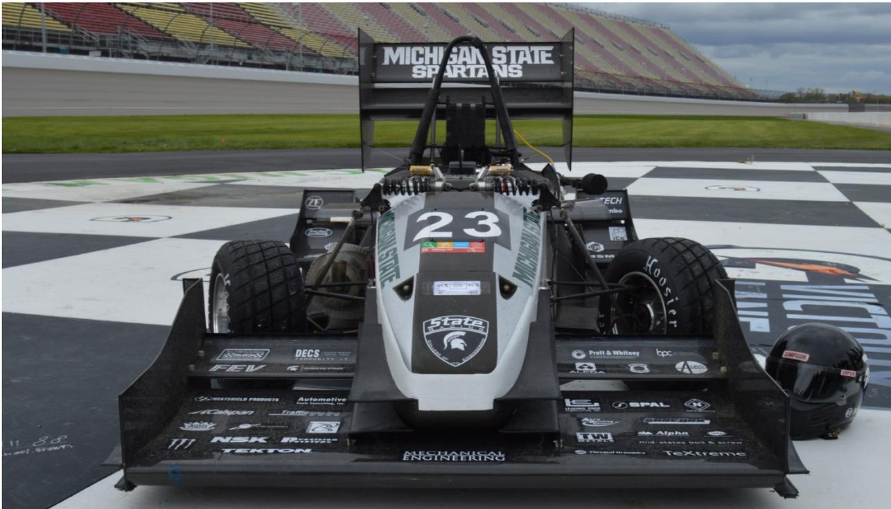
Strain gage sensors from Micro-Measurements<sup>®</sup>, a brand of Vishay Precision Group (VPG), are used by the Michigan State University Formula Racing Team on its 2015-16 season SR-16 car to understand the loading on each of the tires. The acquired data is used to improve suspension tuning for increased cornering performance. Increasing the cornering performance allows for higher corner exit speeds, resulting in faster lap times.
