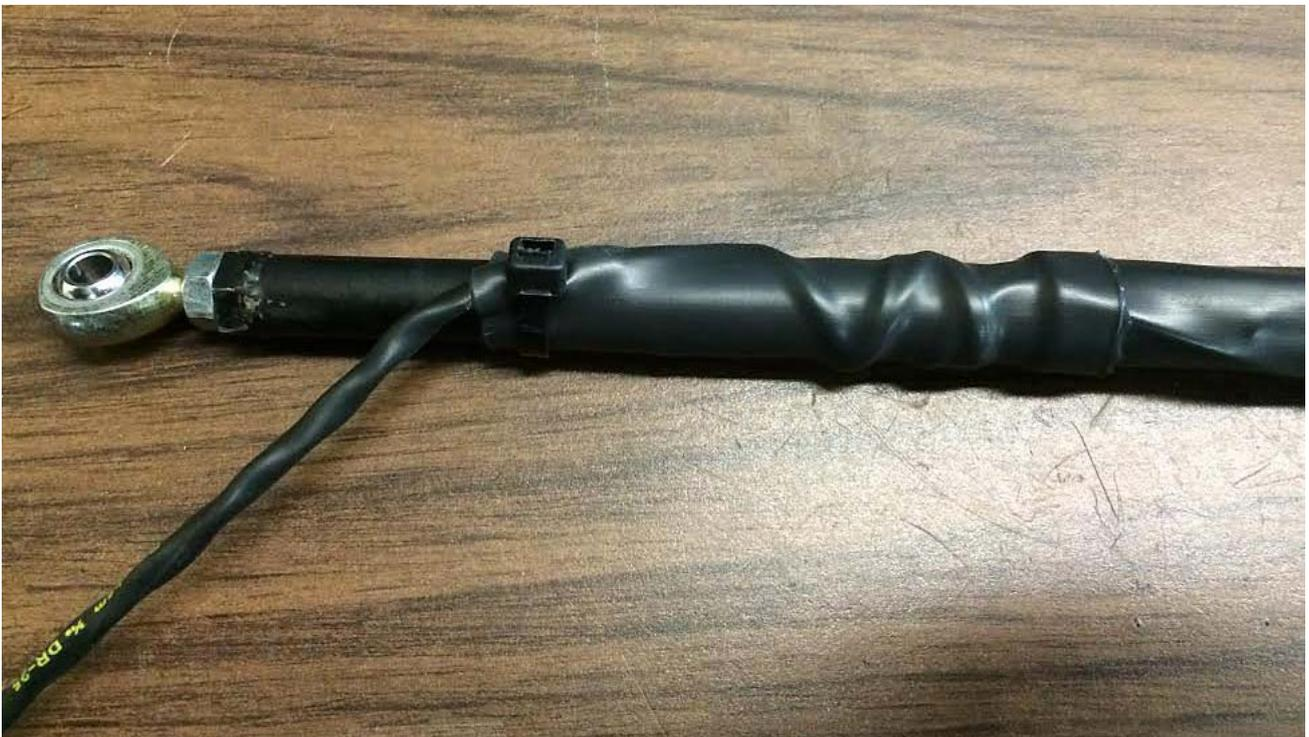
*Figure 1: Completed application of strain gage on pushrod with protective heat shrink over the strain gage sensor*
